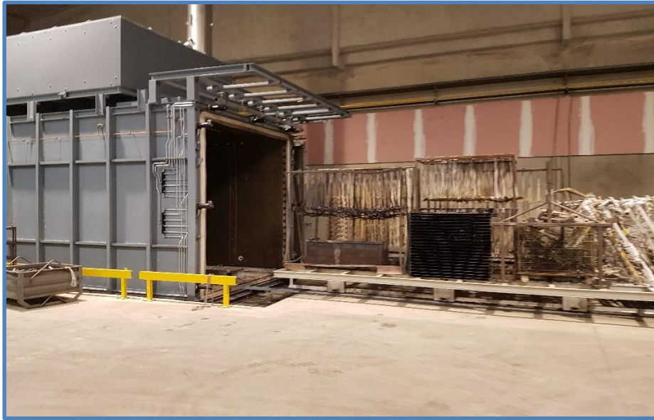
Result of cleaning hooks, hangers etc. after the pyrolysis process
