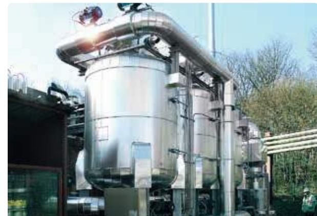
Under specific conditions of high mono- or bi-solvent concentration, the use of activated carbon is suitable for the internal regeneration process after being saturated with organic substances.
