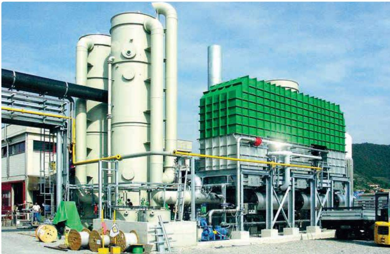
**Airprotech** assures the high destruction efficiency of pollutants in a safe and controlled environment, ensuring an effective combustion chamber temperature and residence time suitable for the complete oxidation of halogenated compounds. In addition, specialized engineering of **Airprotech** plants ensures high reliability and resistance to aggressive substances over time.
