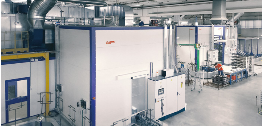
➤ Step-by-step automatic liquid painting system with floor conveyor
