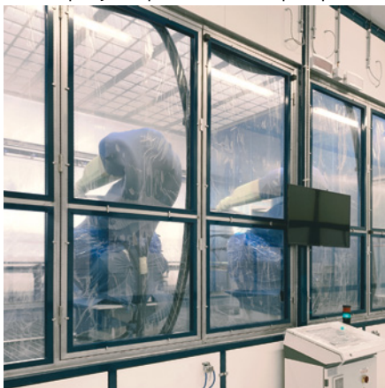
➤ Automatic step-by-step liquid painting system with floor conveyor for automotive applications
