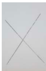
Aluminium | 1 layer powder coating | 1008 hr ASST
