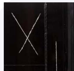
Aluminium | Epoxy + Top Coat | 1008 hr ASST
