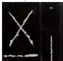
Aluminium | Epoxy + Top Coat | 1008 hr ASST
