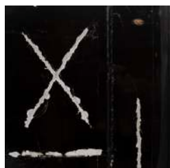
Aluminium | Epoxidharz + Topcoat | 1008 Std ESST
