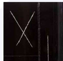
Aluminium | Epoxidharz + Topcoat | 1008 Std ESST
