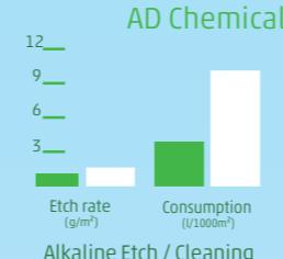
In traditional line set ups the cleaning and etching zone causes several negative side effects a.o.; more contamination in subsequent process steps and the formation of sludge which leads to unnecessary amounts of waste water. The AD Chemicals process has optimized etching steps which improves (waste-) waterflow.
