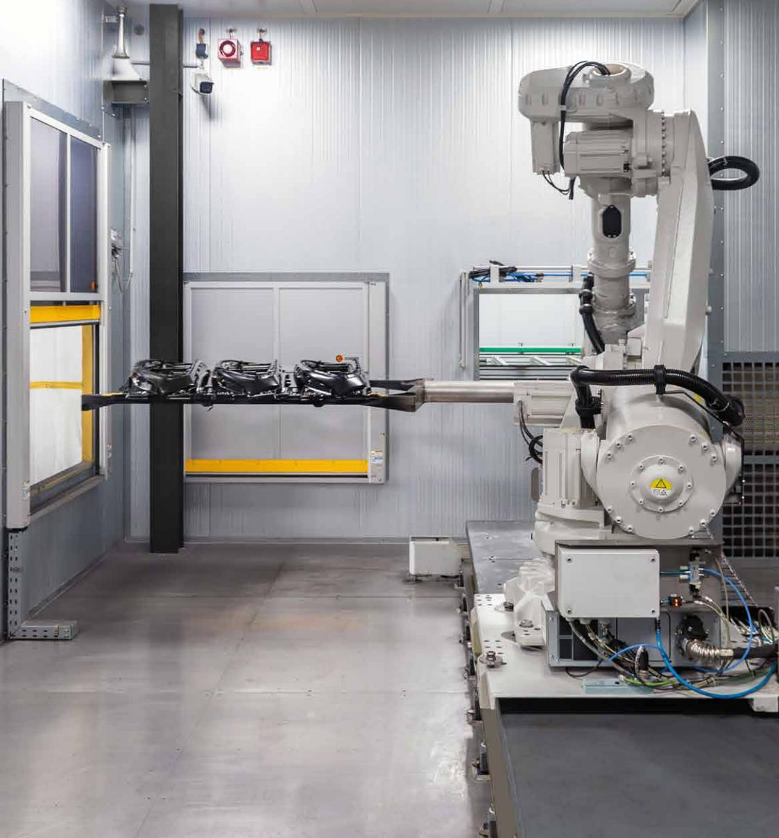
There is often little space in existing building structures for the integration of a complex coating system. This is where our Smart Compact Painting Line concept comes in. Unlike conventional continuous systems, the RIPPERT Smart Compact Painting Line allows for individual system configuration. Various pre-treatment options such as CO<sub>2</sub> cleaning, plasma, flaming and ionisation can be integrated into this modular concept.
