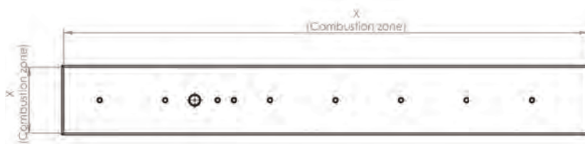
Generic drawing of a typical flat rectangular Eratec gas infrared emitter
