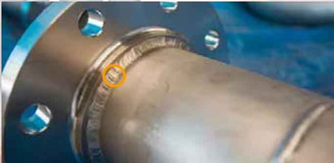
Determining of the ferrite and martensite content of weld seams
