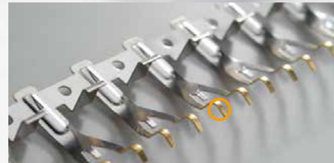
Quality control of galvanized plug contacts
