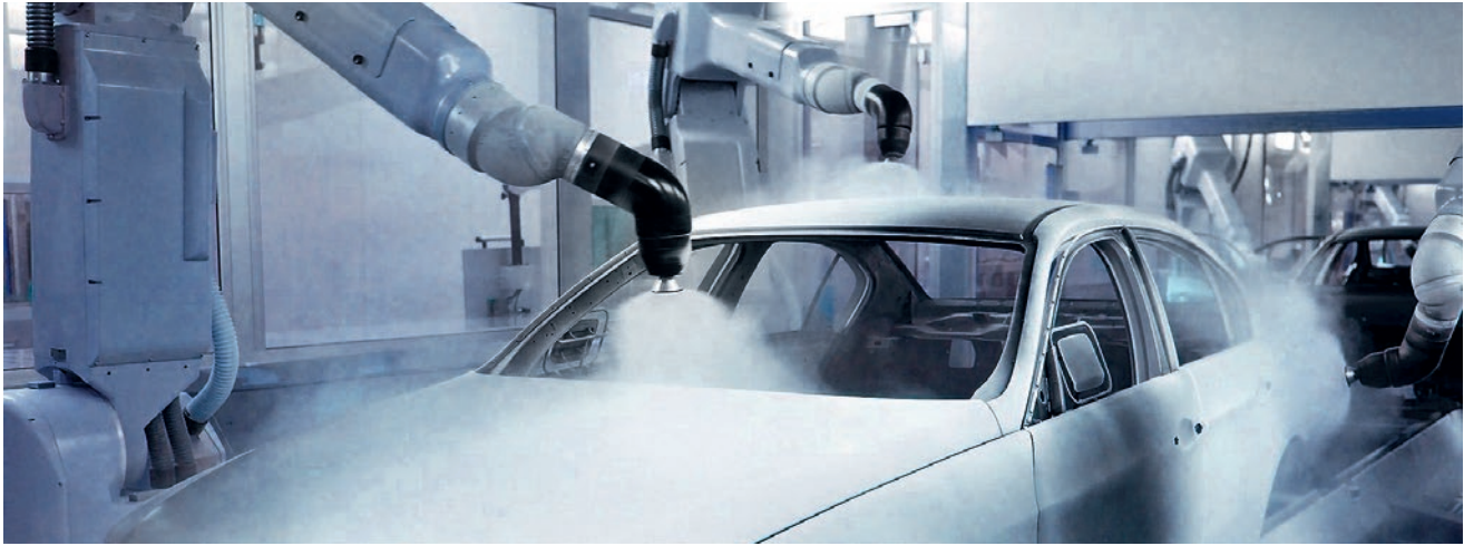
Demand-optimized supply air filtration reliably prevents paint inclusions and thereby minimizes painting costs.
