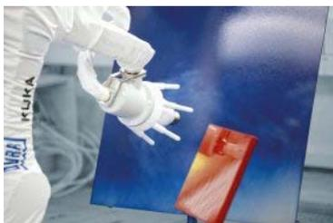
The ready-to-use compact robot, equipped with ultramodern application technology which is matched to the respective application, was specially developed for automated paint application for general industrial use.
