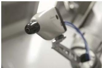
Application efficiency for liquid painting can be significantly increased with the help of new electrostatic spray guns.
